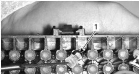
1. Seal out of its cavity - TYPICAL
