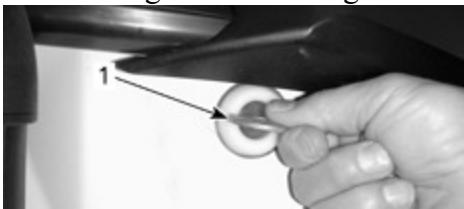
typical - Tightening of fitting
