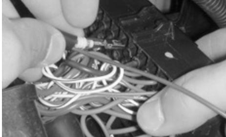
NOTE: Terminal locations have different orientations depending on their position in the fuse box. When inserting the terminals in their respective locations, make sure to follow the orientation of the cavity. When the terminals are inserted correctly, they will "click-in". Verify that the terminals are properly locked in by pulling back on the wire.
