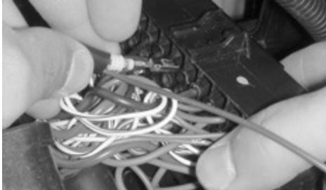
NOTE: Terminal locations have different orientations depending on their position in the fuse box. When inserting the terminals in their respective locations, make sure to follow the orientation of the cavity. When the terminals are inserted correctly, they will "click-in". Verify that the terminals are properly locked in by pulling back.
