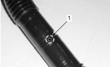
1. Vent hole positioned upwards
